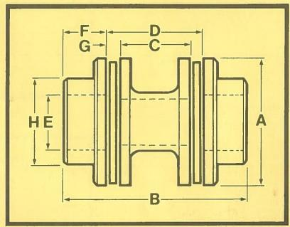
Dimensions given relate to the standard range and are for design layout only. Hub and spacer lengths can be readily increased to suit requirements.
